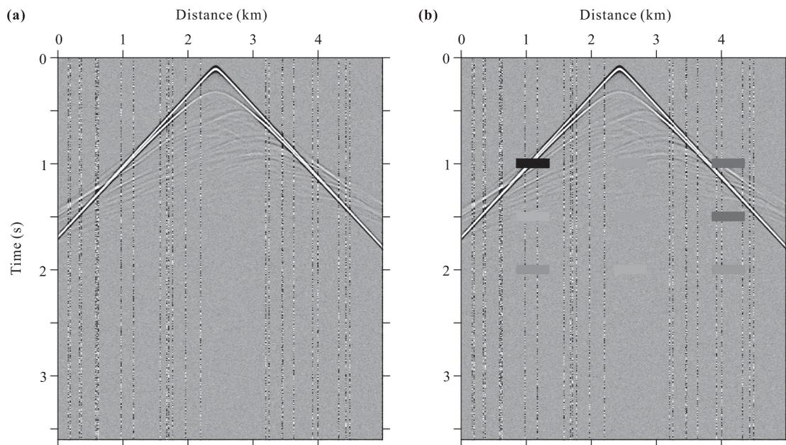
**Figure 13.** Common shot gathers of the 17th shot generated from the Marmousi model. Panel (a) shows the data contaminated by Gaussian white noise with the signal-to-noise ratio (SNR) of 20 dB, where the seismic traces have been randomly rescaled by a factor 20 to simulate strong ground motion. Panel (b) shows the data contaminated by non-Gaussian noise generated by adding up to nine rectangles in whose interior the data are first replaced by its average value and then rescaled by a factor 20.
