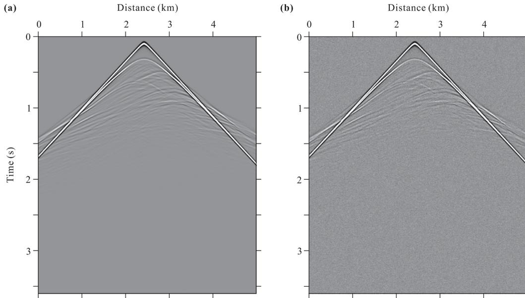
**Figure 7.** Common shot gathers of the 17th shot generated from the Marmousi model, without and with Gaussian white noise: (a) noise-free data; (b) data contaminated by Gaussian white noise with signal-to-noise ratio (SNR) of 20 dB.
