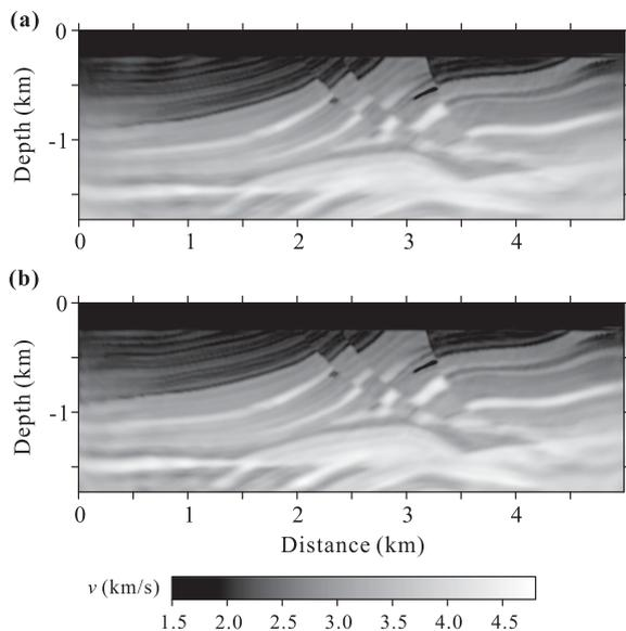
**Figure 11.** Multiscale images obtained using arbitrarily rescaled data (by applying the scalars indicated in Fig. 10) and the normalized zero-lag cross-correlation function. The initial model is shown in Fig. 6(b). Panel (a) is the result obtained with the rescaled noise-free data (reference Fig. 7a). Panel (b) is the result obtained with the rescaled data contaminated by Gaussian white noise with low signal-to-noise ratio (SNR) of 20 dB (reference Fig. 7b).
