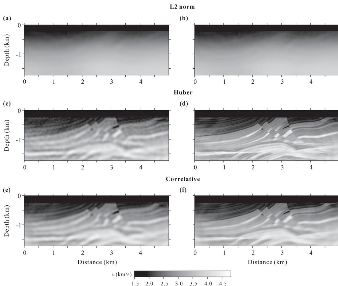
**Figure 14.** Multiscale images obtained by FWI with different objective functions. The initial model is shown in Fig. 6(b). From top to bottom, inverted results computed at two frequency bands with the L2 norm (a and b), the Huber norm (c and d) and the normalized zero-lag cross-correlation function (e and f). Here, the data is contaminated by Gaussian white noise (SNR equal to 20 dB) and some traces are rescaled by a factor 20 (Fig. 13a).
