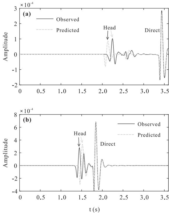
**Figure 19.** The observed (solid black lines) and predicted (dashed grey lines) data excited by the two shots shown in Fig. 6 and recorded at the last receiver (the triangle). The plot (a) shows the data from the first shot, while the plot (b) shows the data from the 17th shot. The head and direct waves are indicated in both plots.
