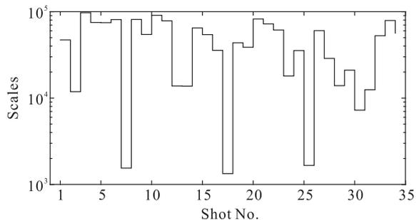
**Figure 10.** Scalars that were used to arbitrarily rescale 34 shot gathers synthesized from the Marmousi model.
