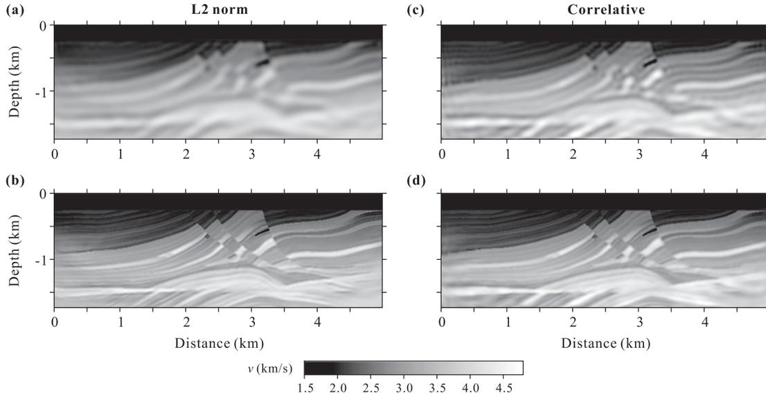
**Figure 8.** Multiscale images obtained using noise-free data (Fig. 7a) and two different objective functions. The initial model is shown in Fig. 6(b). The left-hand column are the results obtained by the conventional L2 norm at two frequency bands (from low to high frequency bands, a and b), while the right-hand column are the results obtained with the normalized zero-lag cross-correlation function at the same frequency bands (from low to high frequency bands, c and d).
