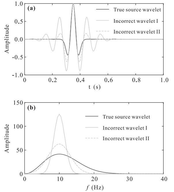
**Figure 2.** Source wavelets in time-domain (a) and frequency domain (b). The solid black lines represent the true wavelet, while the solid and dashed grey lines represent the two incorrect source wavelets, respectively.
