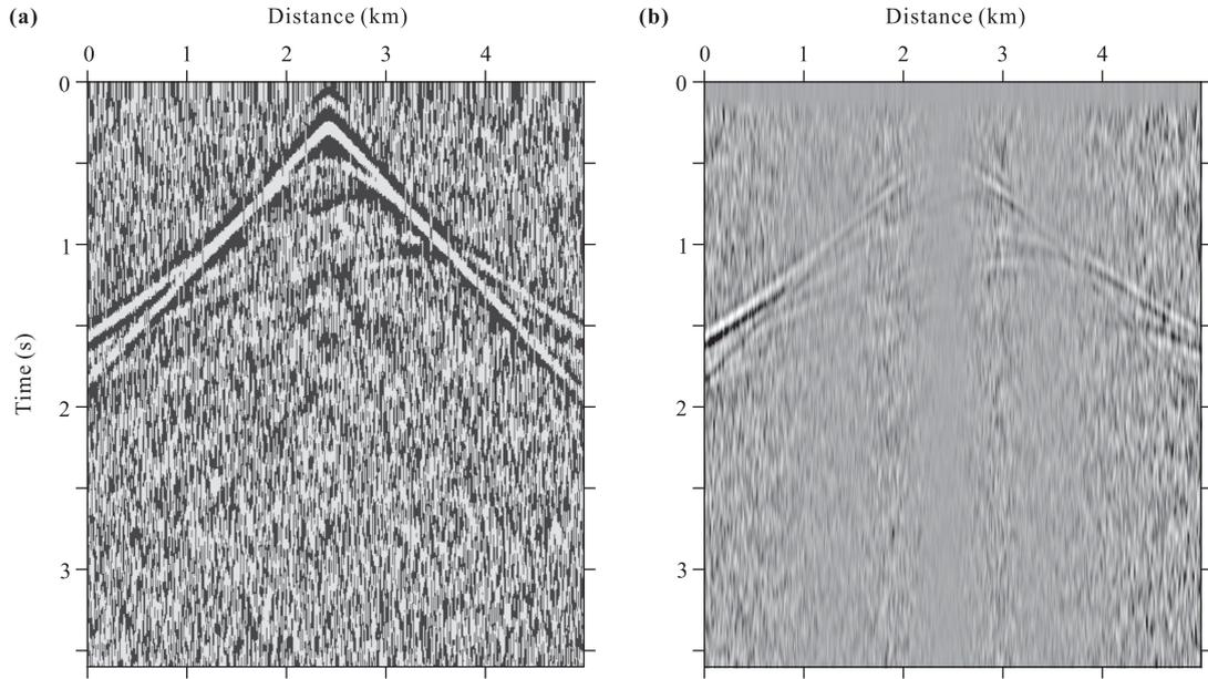
**Figure 15.** The initial adjoint sources of the 17th shot generated from the rescaled traces shot gathers (Fig. 13a) and different objective functions. Panel (a) shows the initial adjoint source obtained by the Huber norm, while panel (b) shows the initial adjoint source obtained by the normalized zero-lag cross-correlation function.
