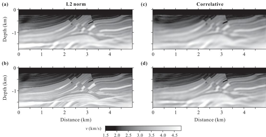
**Figure 20.** Multiscale images obtained using noise-free data (Fig. 7a) and two different objective functions. The initial model is shown in Fig. 6(c). The left-hand column shows the results obtained by the conventional L2 norm at two frequency bands (from low to high frequency bands, a and b), while the right-hand column shows the results obtained with the normalized zero-lag cross-correlation function at the same frequency bands (from low to high frequency bands, c and d).
