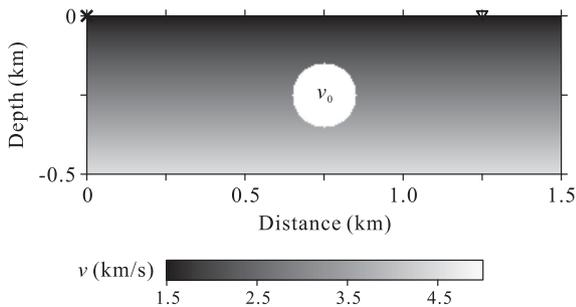
**Figure 1.** A 2-D canonical model integrated by a medium where the velocity increases vertically from  $1.5 \text{ km s}^{-1}$  at surface to  $4.5 \text{ km s}^{-1}$  at the bottom, and a buried spherical-shaped body (circular in the plane) that has a radius of 0.15 km and seismic velocity  $v_0 = 5.0 \text{ km s}^{-1}$ . On top, the cross denotes the first shot point, while the triangle denotes a receiver.
