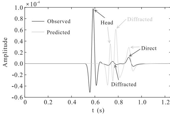
**Figure 5.** The observed (solid black line) and predicted data (dashed grey line) excited by the first shot shown in Fig. 1 and recorded at the receiver (the triangle). The head, diffracted and direct waves are indicated.
